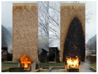
A fire test of the shingle facade
