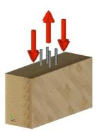
Glued-in threaded rods are used in construction to replace conventional fasteners. The load-bearing capacity of various standard connections was investigated. Characteristic values were determined from the test results.
