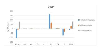
The use of sustainable building products is increasingly in demand. As a result, three conventional ceiling structures were compared with regard to their life cycle assessment on the basis of various standards. This resulted in a calculation table for the evaluation of different building components in terms of their life cycle assessment.
