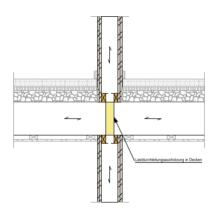
Detail load transmission apartment partition wall
