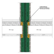
Detail load transmission inside wall
