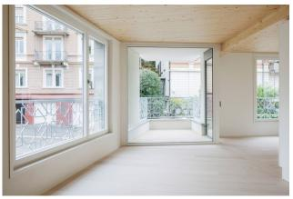
In the middle of a Zurich villa district, an apartment building was constructed exclusively of wood. Thanks to the timber construction method, the four apartments of the new building were ready for occupancy within one year from the start of construction.
