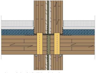
Load transmission detail with beech dowel
