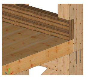
Visualization Cadwork - support on trusses
