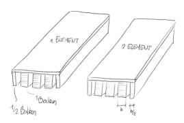
An element is made of 3 joists and 2 half-joists.
