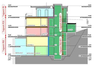
Section with the different fire sections
