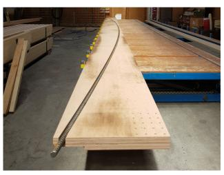
In detail: fish-bellied pre-stressing bar milled into the beech girder
