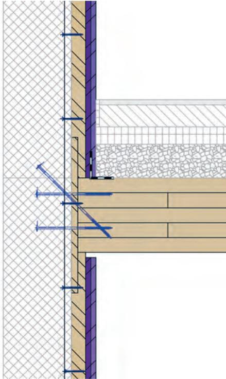
The timber structures serve as a lost shuttering for the concrete. This way we saved time, 1270 tons of concrete and 24 tons of steel.
